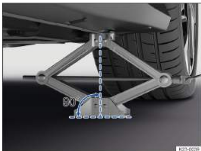
Fig. 3 At the rear left-hand side of the vehicle: jack applied.
