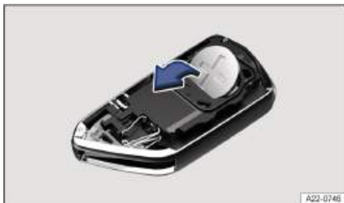
Fig. 2 Vehicle key: replacing the button cell.
