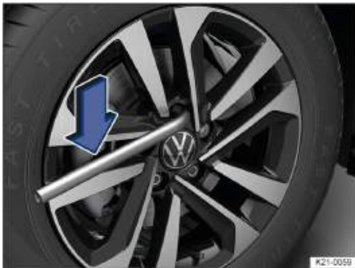
Fig. 1 Loosening wheel bolts.
