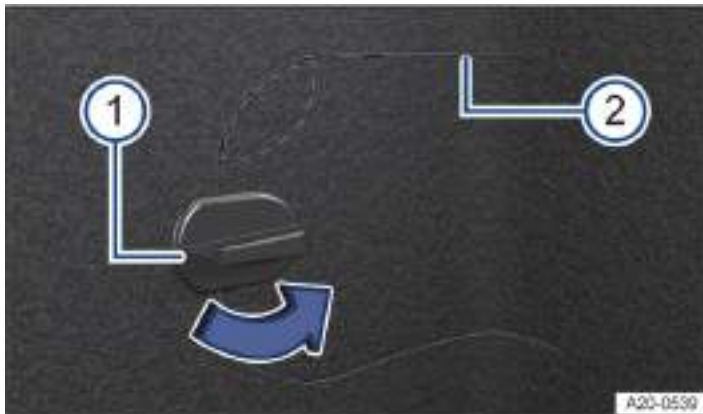
Fig. 1 In the lower right-hand side of the luggage compartment trim: flap for the manual release (illustration).
