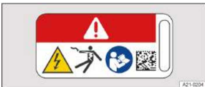
Fig. 2 Warning sign on high-voltage components.
