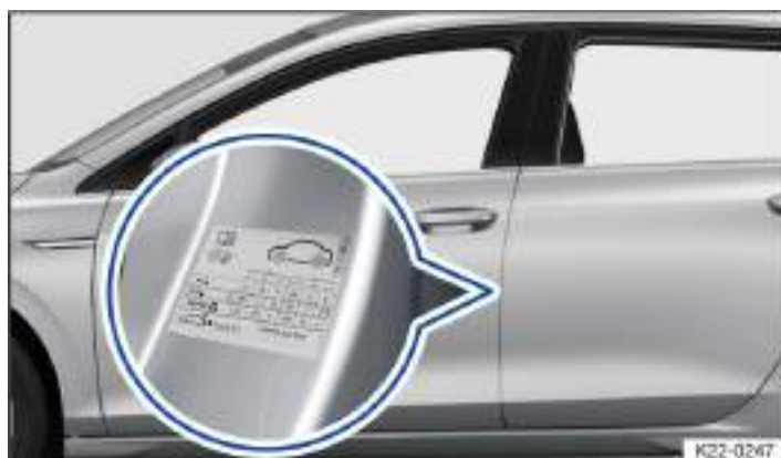
Fig. 2 On the driver door pillar: tyre pressure sticker (alternatively on the inside of the charging socket flap)
