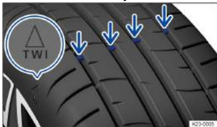
Fig. 1 In the tread grooves: tread wear indicator.
