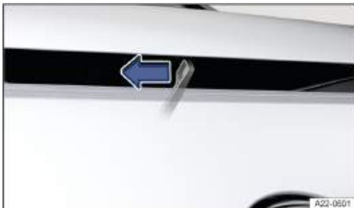
Fig. 2 On the bonnet: control lever.
