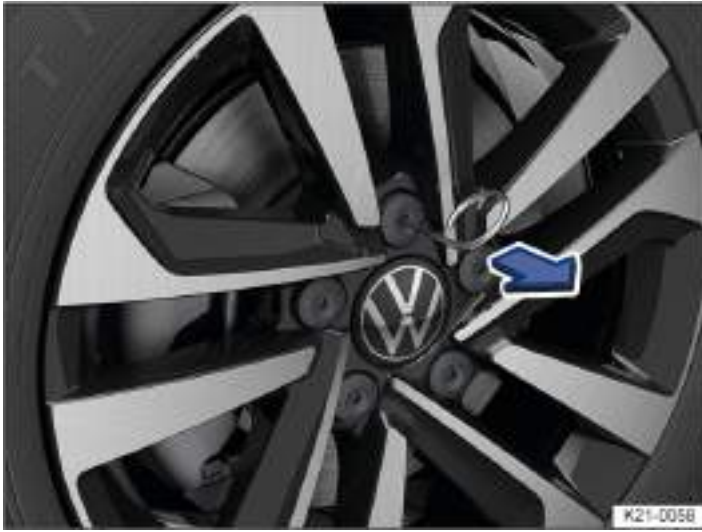
Fig. 1 Removing the wheel bolt caps.
