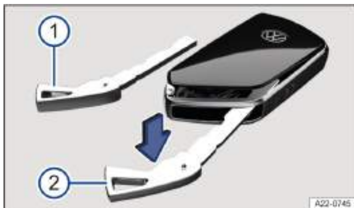
Fig. 1 Vehicle key: opening the battery compartment cover.
