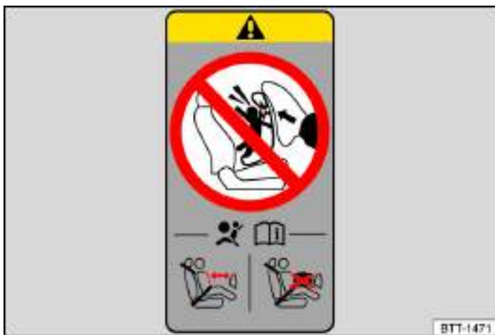
Fig. 2 On the B-pillar: airbag label(illustration).
