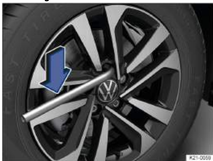
Fig. 1 Unscrew the wheel bolts with the wheel wrench.
