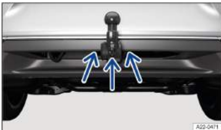
Fig. 1 On the towing bracket: eye for securing the safety or breakaway cable (illustration).
