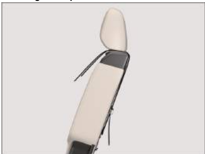
Fig. 3 On the rear of the outer seats of the rear bench seat or front passenger seat: attached top tether.
