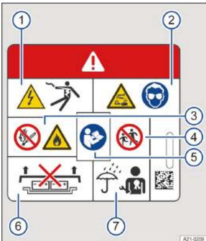
Fig. 5 Warning sign on high-voltage battery.
