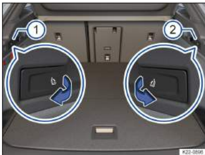
Fig. 2 In the luggage compartment: remote release lever for the left ① and the right ② parts of the rear seat backrest.
