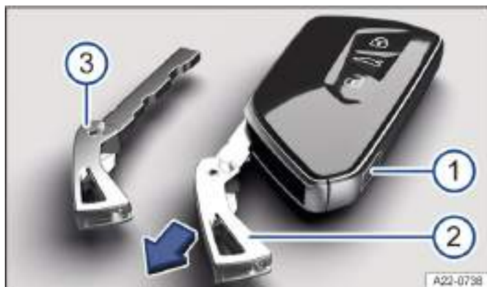
Fig. 1 Vehicle key: releasing the manual key.
