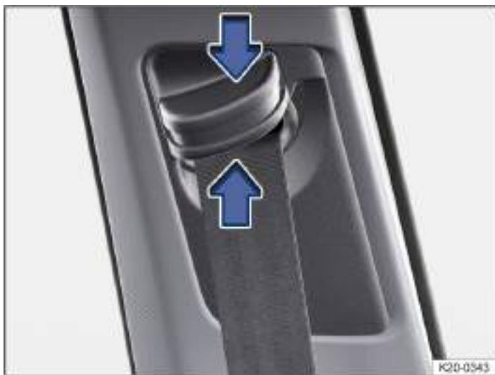
Fig. 1 Next to the front seats: seat belt height adjuster.
