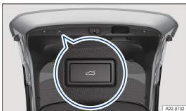
Fig. 2 In the open boot lid: button for electrically closing the boot lid (illustration).
