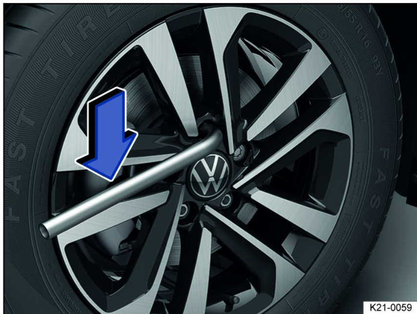
Fig. 197 Wheel change: removing wheel bolts with the lug wrench.
