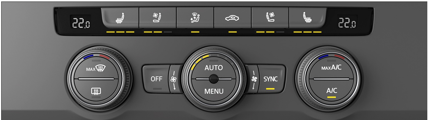
Fig. 92 In the upper section of the center console: air conditioning block for the Climatronic system (version 2).
