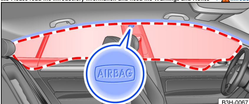
Fig. 30 On the left side of the vehicle: installation location and deployment zone of the Side Curtain Protection®.
