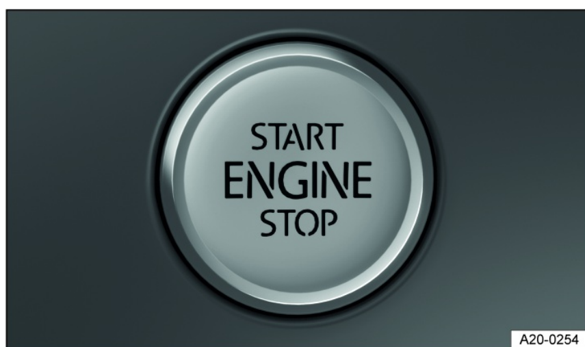
Fig. 95 In the lower area of the center console: starter button for starting the engine.
