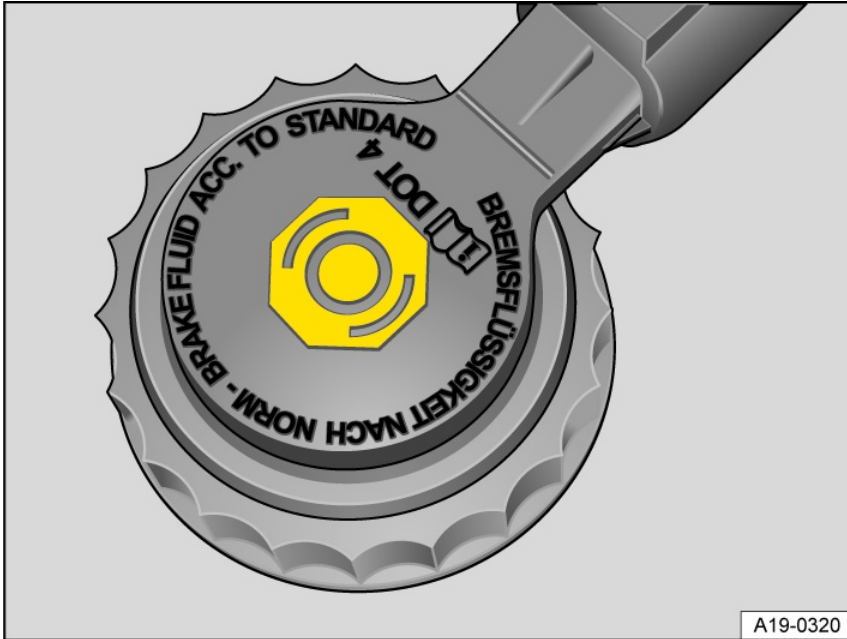
Fig. 176 In the engine compartment: cap on the brake fluid reservoir (version 1).
