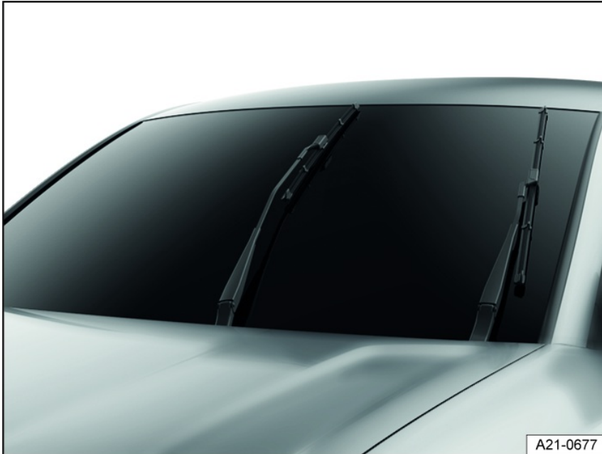
Fig. 151 Windshield wipers in service position (general example).
