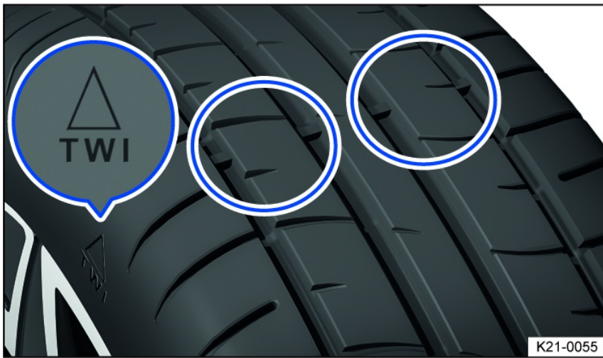
Fig. 181 Tire tread: tread wear indicator.
