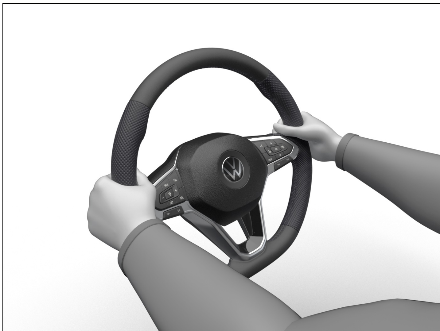
Fig. 67 On the steering wheel: nine o'clock and three o'clock position.
