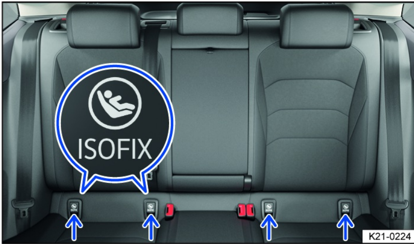
Fig. 36 On the outer seats in the rear bench seat: Designation of the ISOFIX/lower LATCH anchorage points for child restraints.
