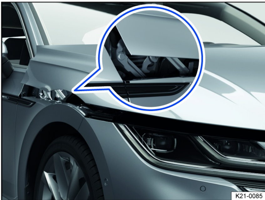
Fig. 44 Triggered re-active hood (general example).
