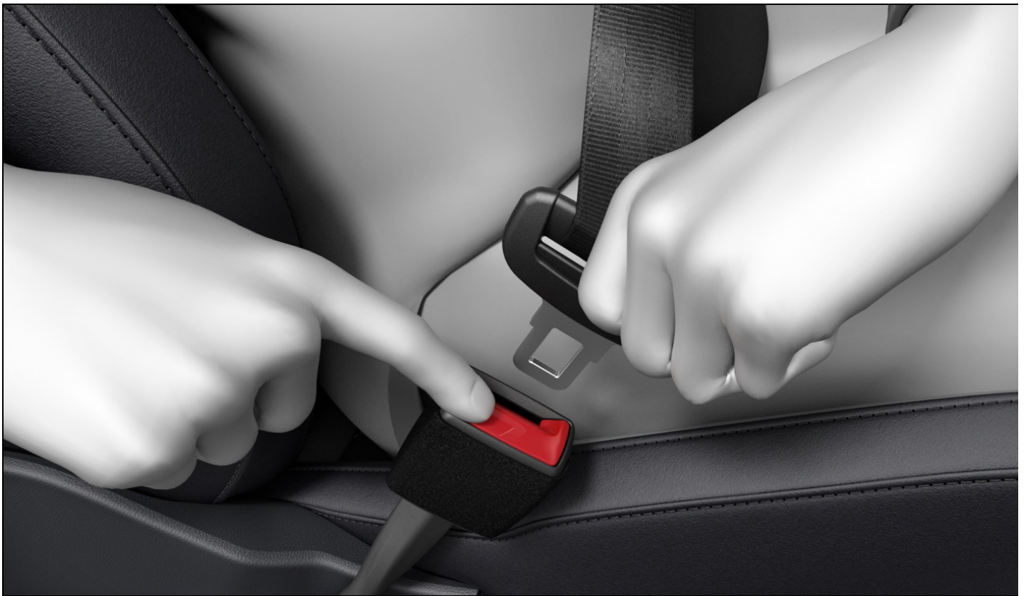
Fig. 21 Releasing the buckle tongue from the safety belt buckle.
