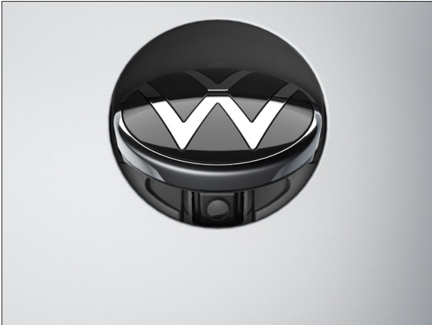
Fig. 201 In the rear of the vehicle: Rear View Camera system in the Volkswagen emblem (general example).
