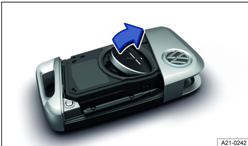
Fig. 50 Vehicle key: replacing the button cell battery
