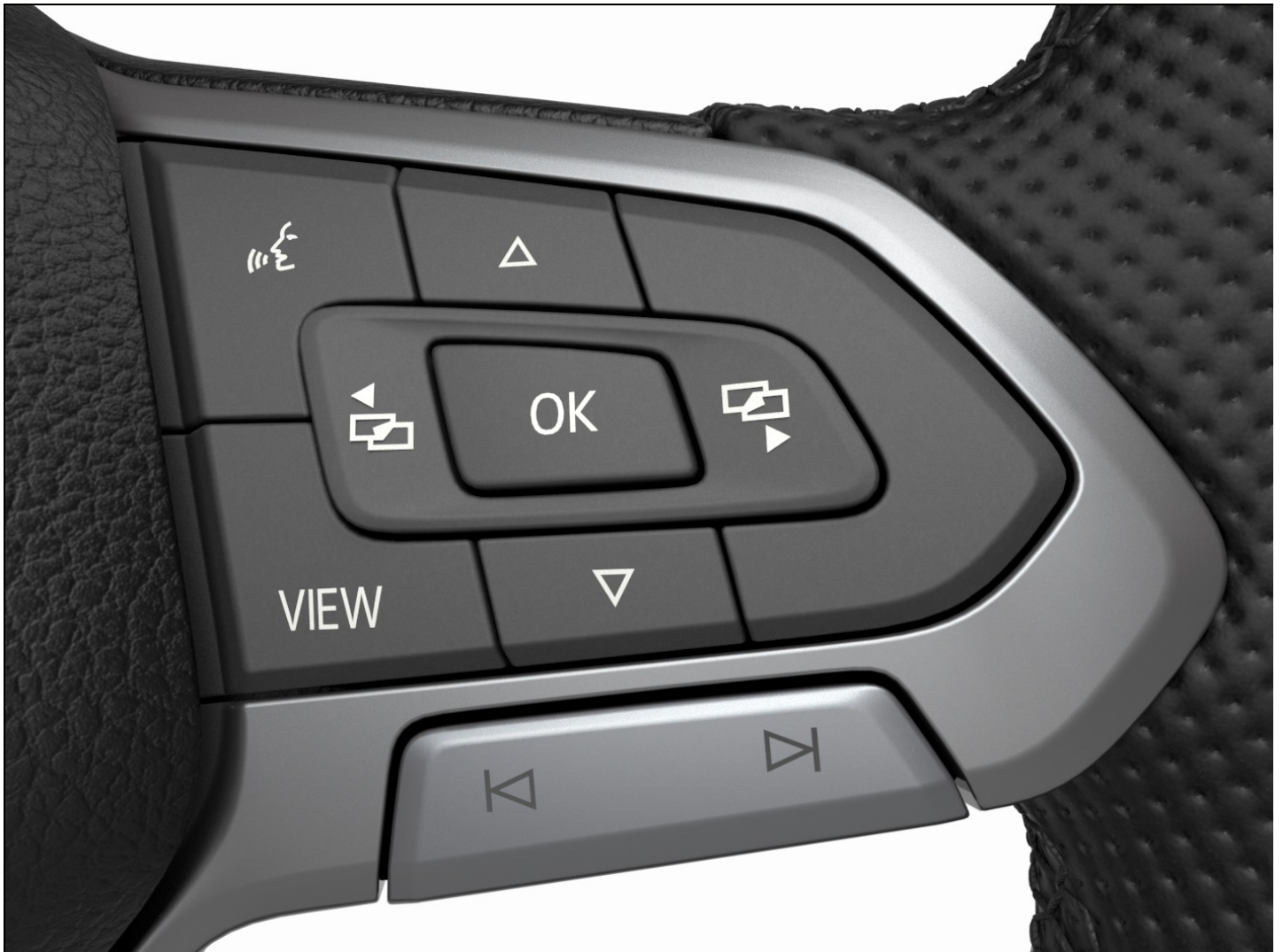
Fig. 10 Right side of the multi-function steering wheel: Operating the Volkswagen Digital Cockpit Pro (variant 1).
