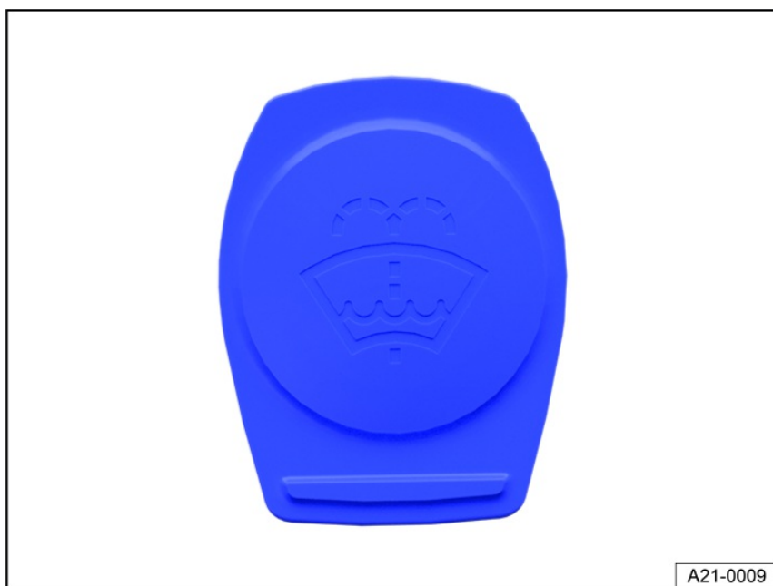
Fig. 171 In the engine compartment: Cap on the washer fluid reservoir (general example).
