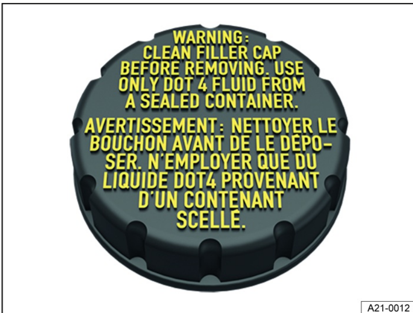
Fig. 177 In the engine compartment: cap on the brake fluid reservoir (version 2).
