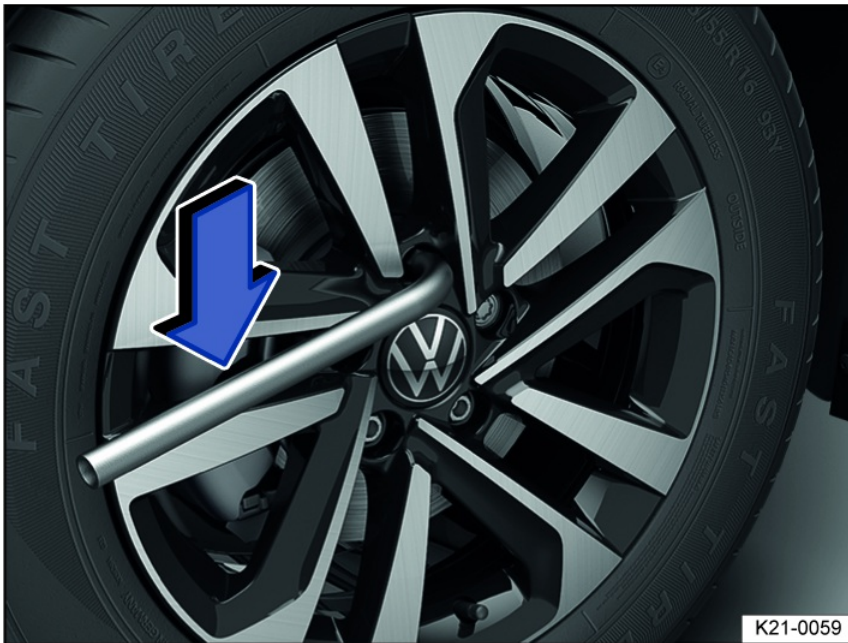
Fig. 186 Changing a tire: loosening the wheel bolts.
