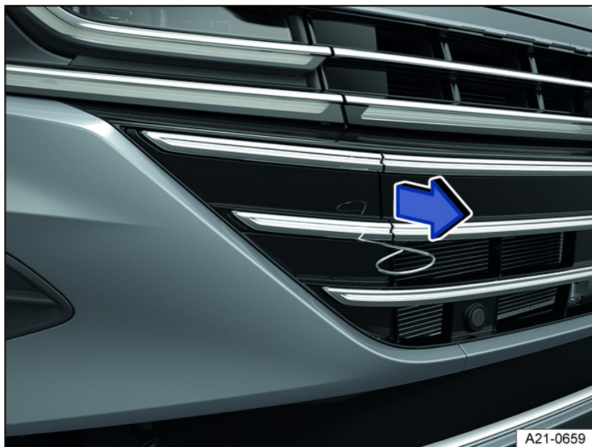
Fig. 164 In the right front bumper: Remove cover.
