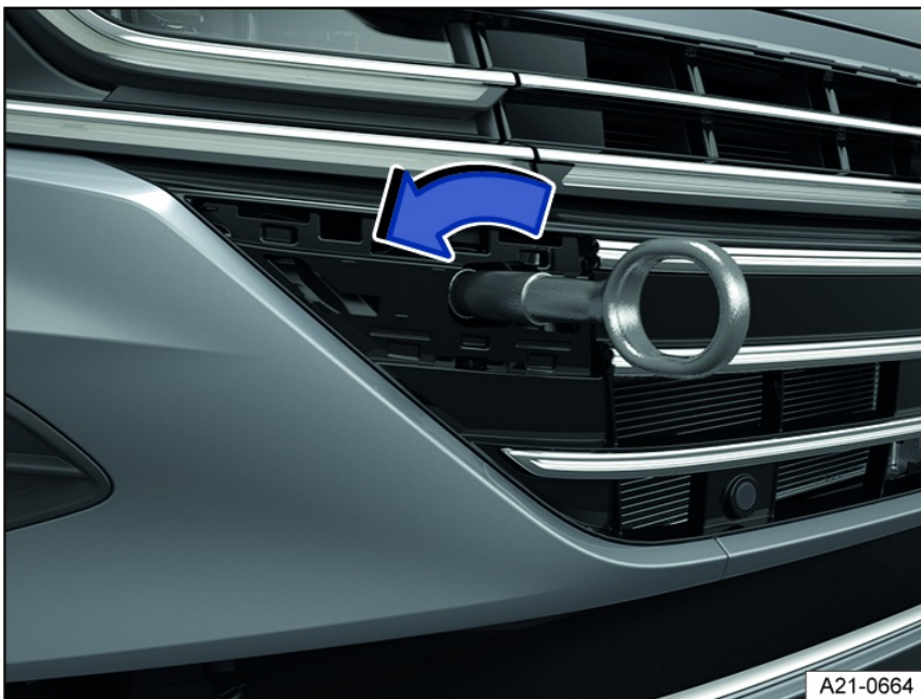
Fig. 165 In the right front bumper: Screw in towing eye.
