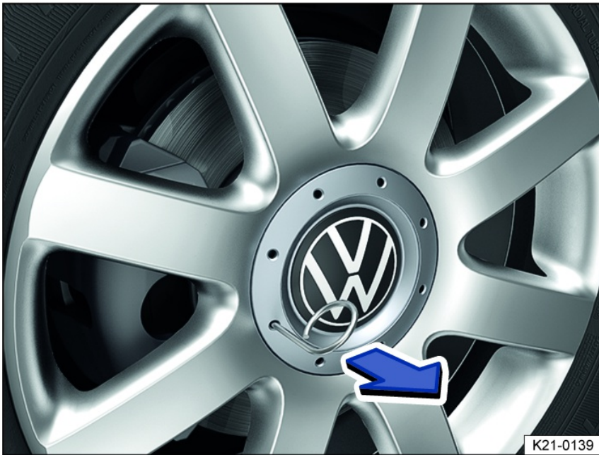
Fig. 183 Remove the hubcap.
