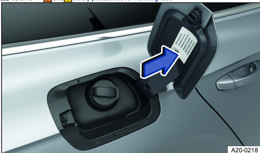
Fig. 148 On the inside of the fuel filler flap: fuel label (general example)
