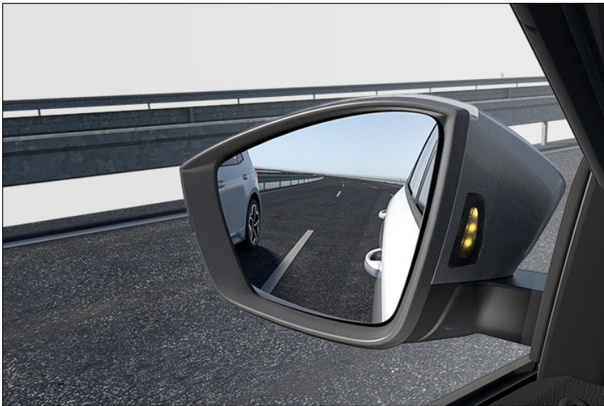
Fig. 118 In the outside mirror housing: Visual indicators for Side Assist.
