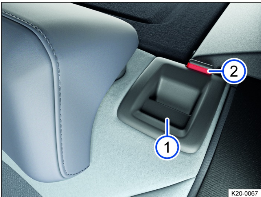
Fig. 71 In the rear seat backrest: release button.
