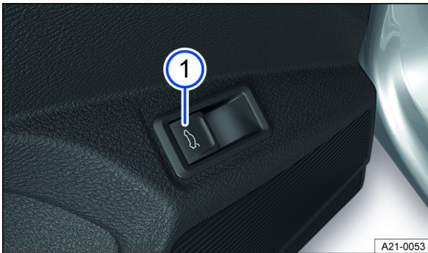
Fig. 54 In the driver's door: Button for powered opening of the trunk lid (general example).
