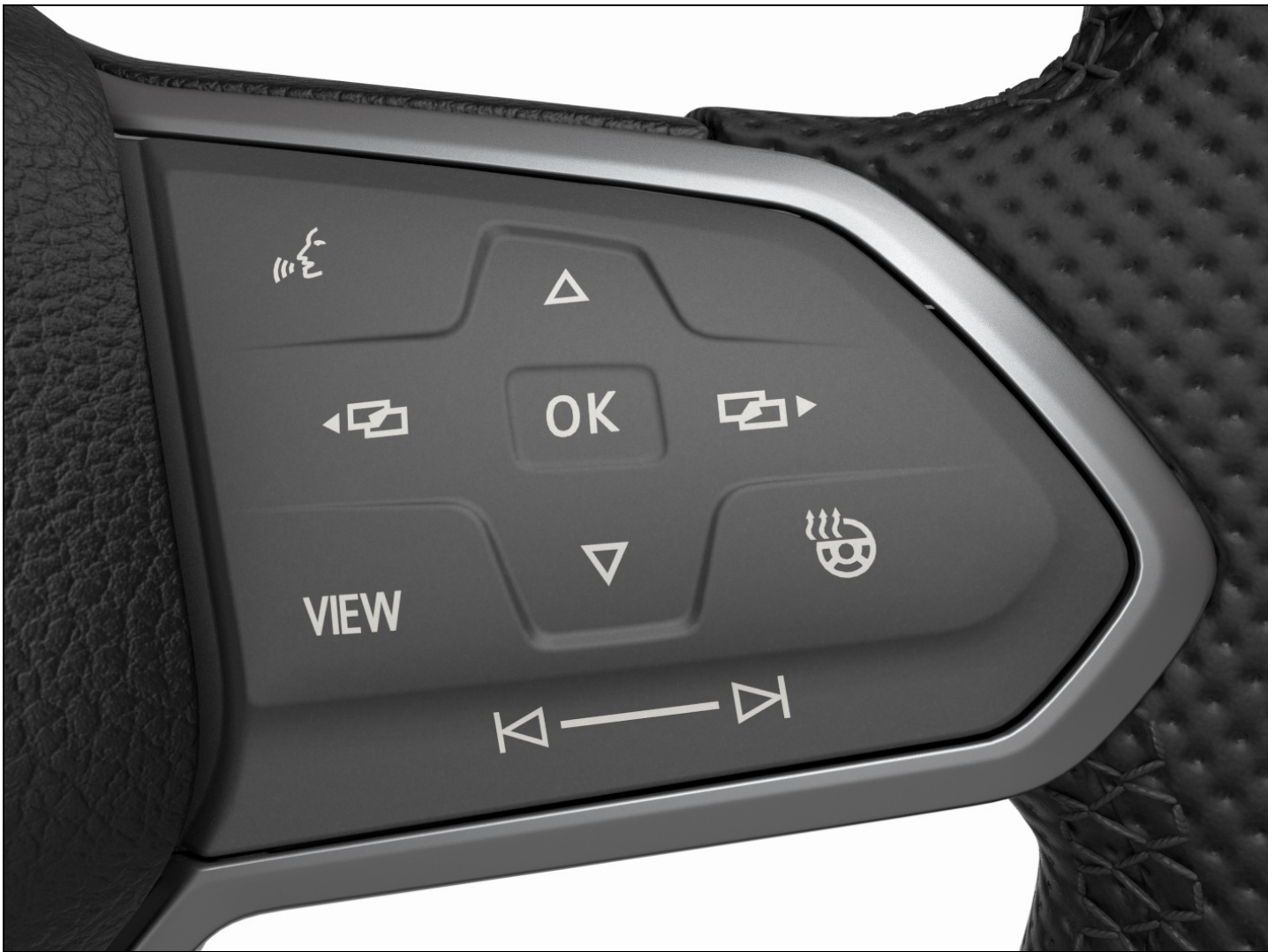
Fig. 11 Right side of the multi-function steering wheel: Operating the Volkswagen Digital Cockpit Pro (variant 2).
