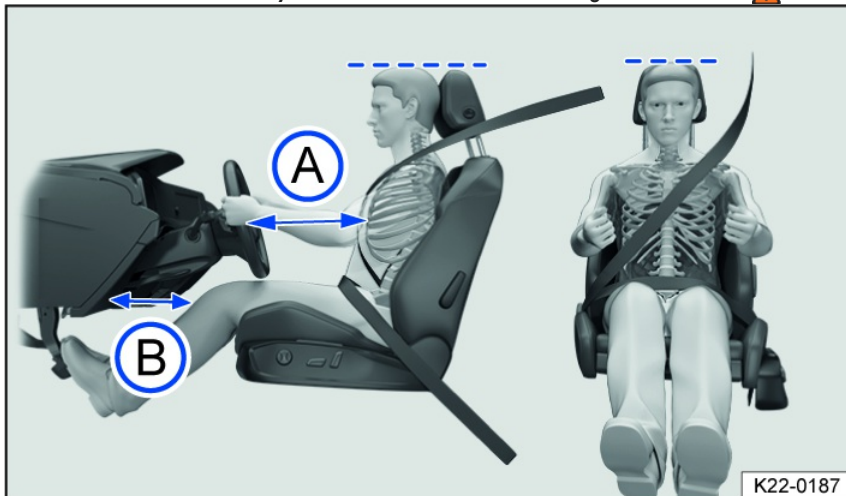
Fig. 18 General example: correct distance between the driver and the steering wheel, correct safety belt routing and correct head restraint adjustment.
