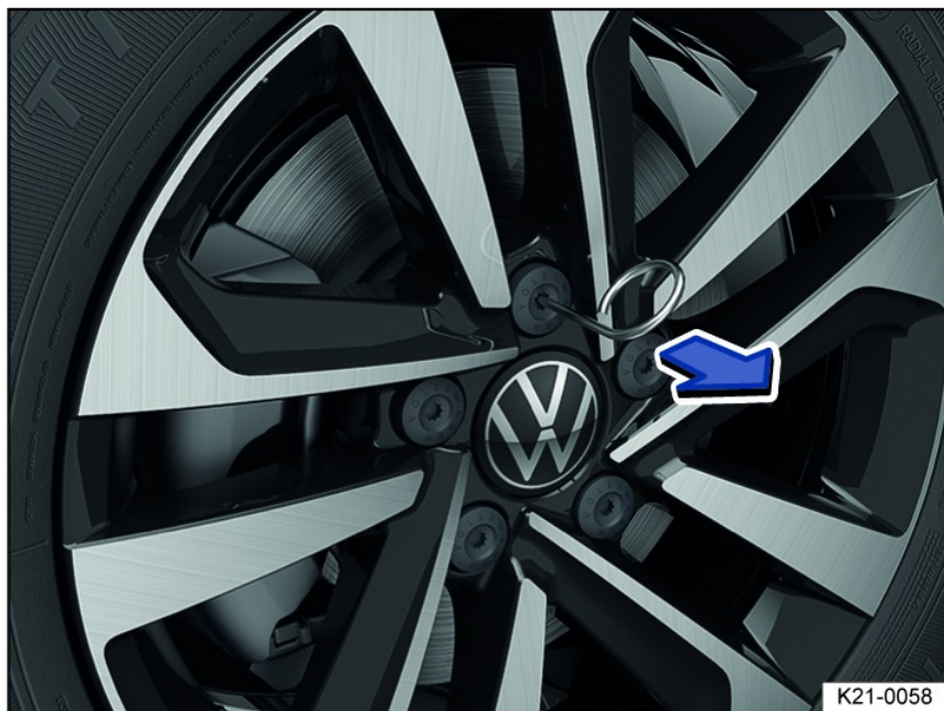
Fig. 185 Remove the caps from the wheel bolts.
