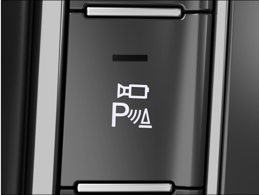
Fig. 125 In the center console: Button for switching the Area View on and off.
