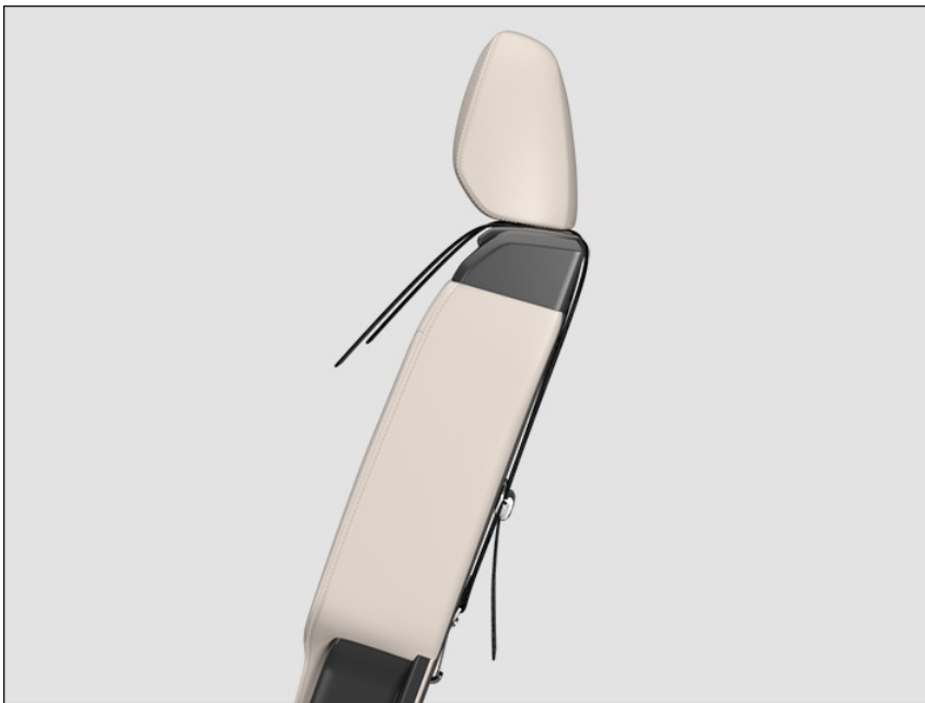
Fig. 39 On the rear side of the outer seats of the second row of seats: Attached top tether safety belt.
