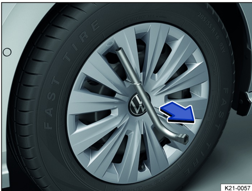
Fig. 184 Remove the wheel hub cover.
