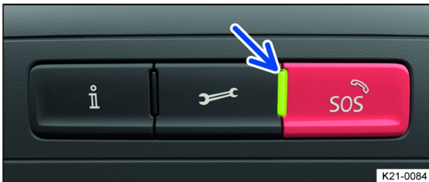
Fig. 45 In the roof console: Controls for call services and indicator light.
