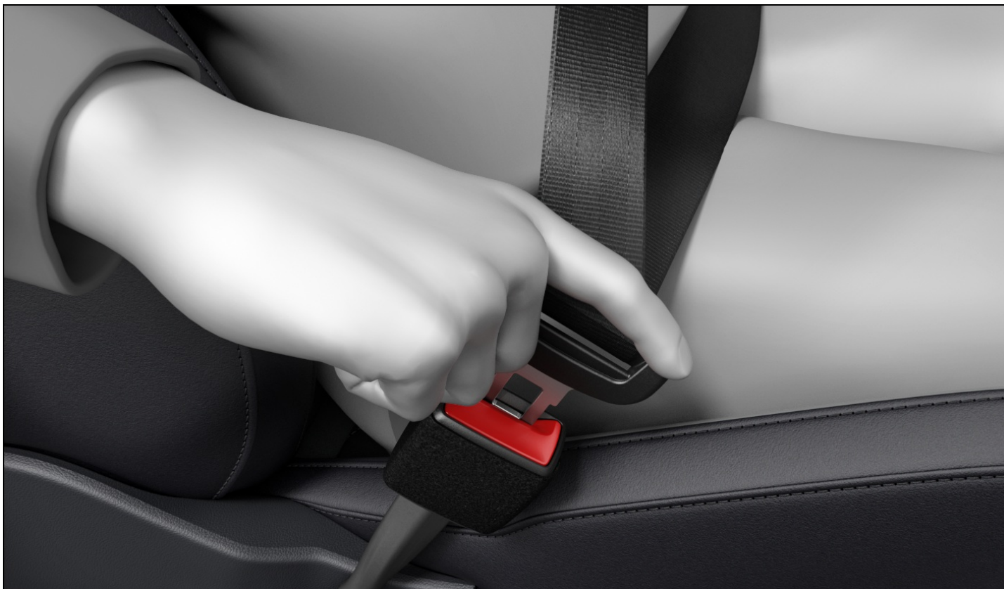
Fig. 20 Inserting the buckle tongue into the safety belt buckle.
