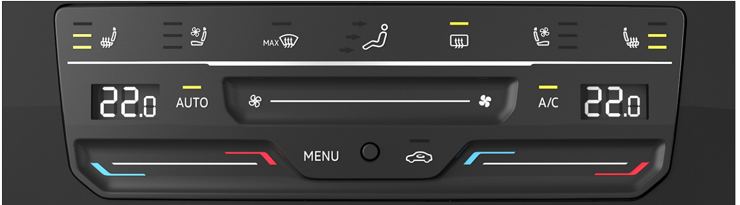
Fig. 91 In the upper section of the center console: air conditioning block for the Climatronic system (version 1).
