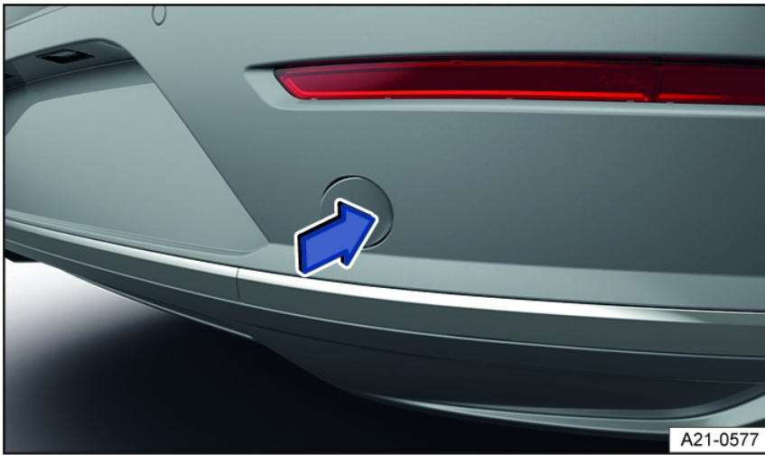
Fig. 166 In the right rear bumper: Remove cover.
