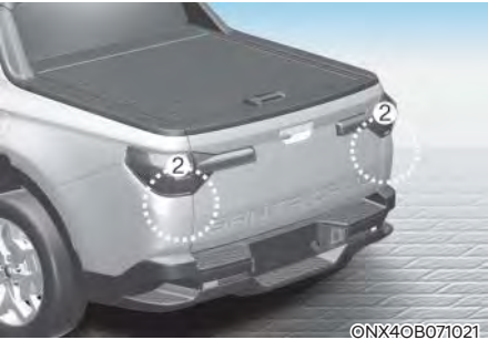
[1] : Front view camera, [2] : Rear corner radar
