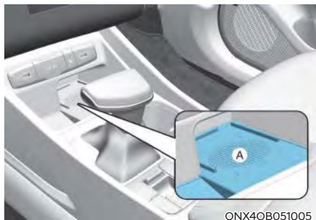
[A] : Wireless Charging Pad (In-vehicle Authentication Pad)
