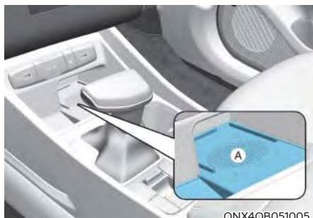
[A] : Wireless Charging Pad (In-vehicle Authentication Pad)
