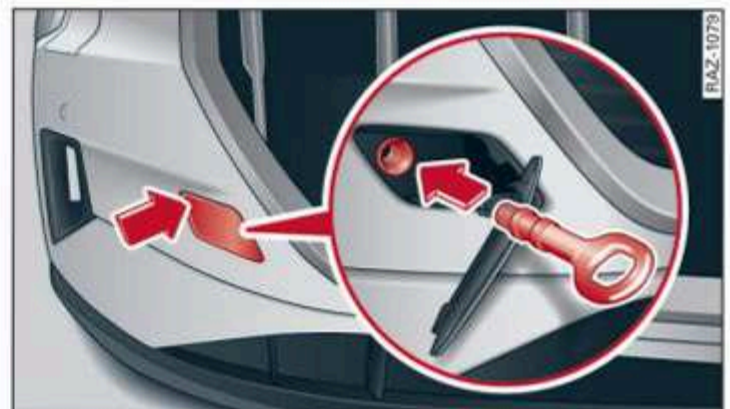
Fig. 180 Front bumper: installing the towing loop
