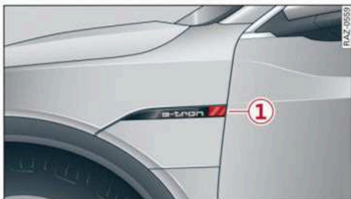
Fig. 86 Left front side of the vehicle: opening the high-voltage charging port door
