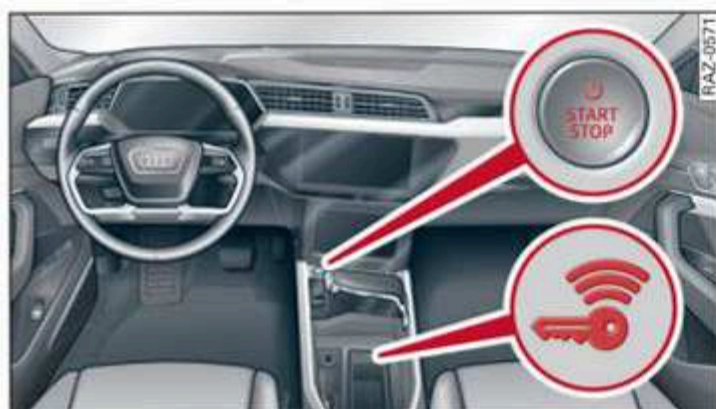
Fig. 82 Center console: switching on the drive system
