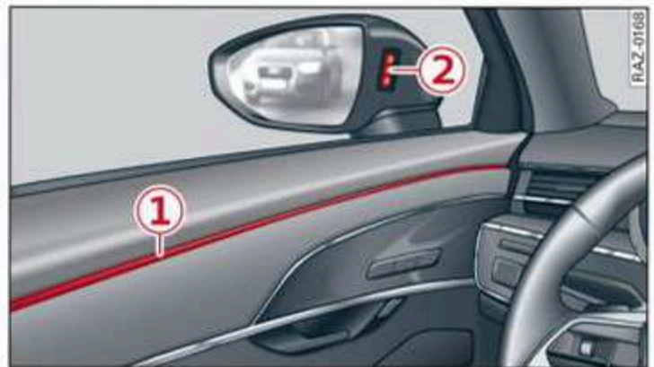
Fig. 122 Front door: warning strip
