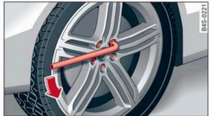
Fig. 175 Wheel: loosening the wheel bolts
