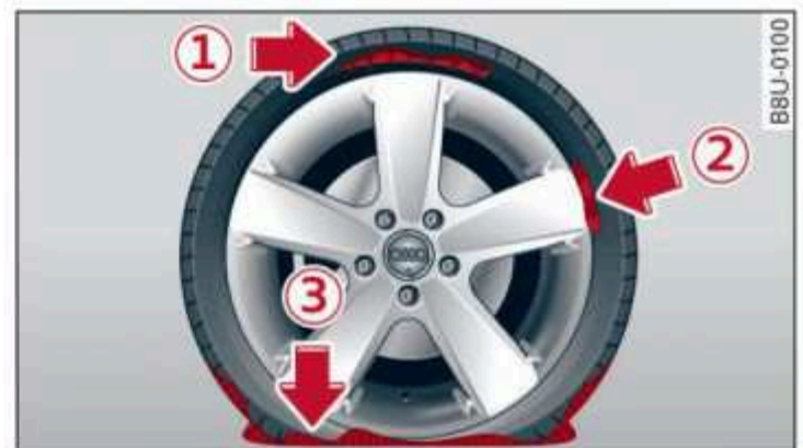
Fig. 170 Tire: tire damage that cannot be repaired
