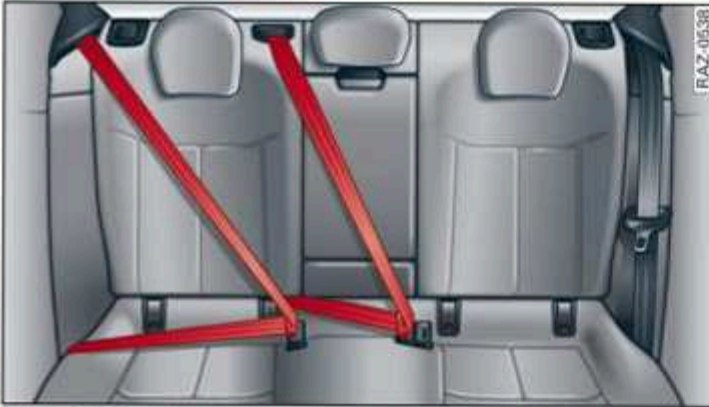
Fig. 67 Rear bench seat: securing unused safety belts
