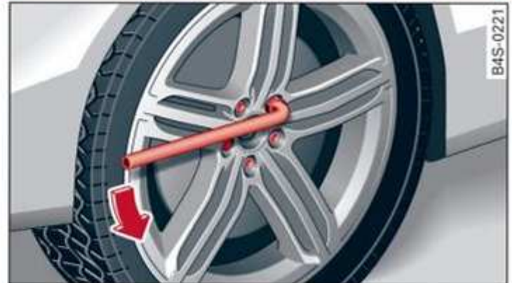
Fig. 175 Wheel: loosening the wheel bolts
