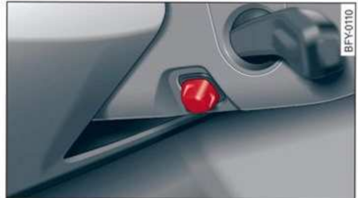
Fig. 54 Steering column: switch for adjusting the steering wheel position
