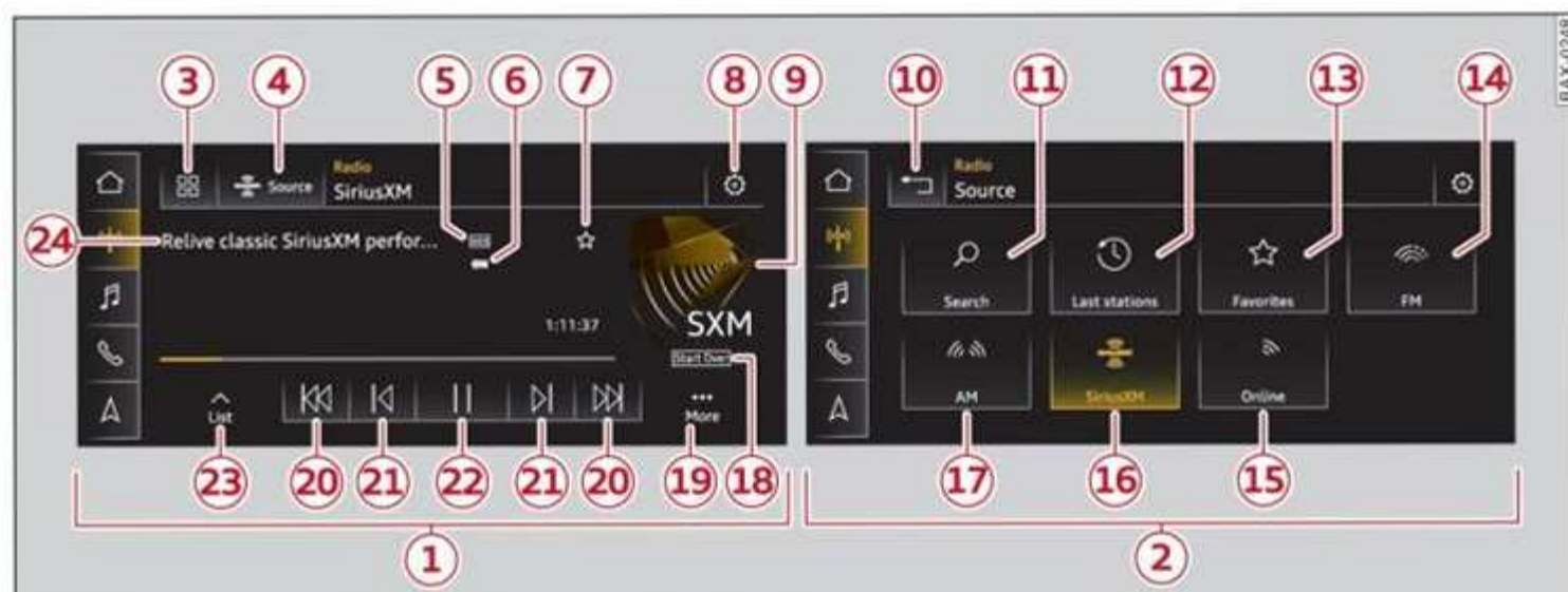
Fig. 150 Upper display: left side: playback view of radio functions, right side: sources
