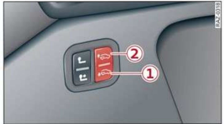
Fig. 74 Left side of the luggage compartment: rear lowering button
