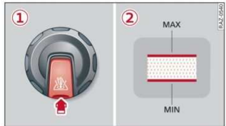
Fig. 161 Engine compartment - Coolant expansion tank (diagram): ① cover with release button; ② markings
