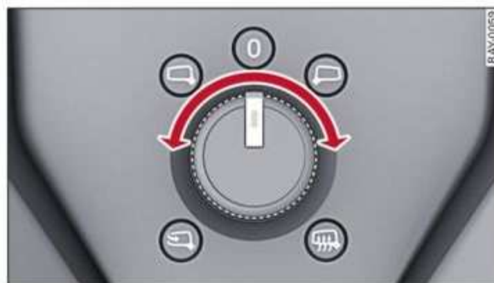
Fig. 40 Driver's door: knob for the exterior mirrors
