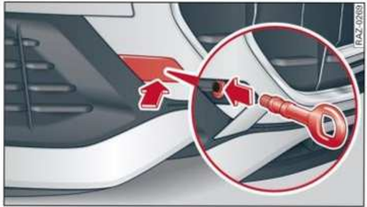
Fig. 182 Front bumper: installing the towing loop (version 1)
