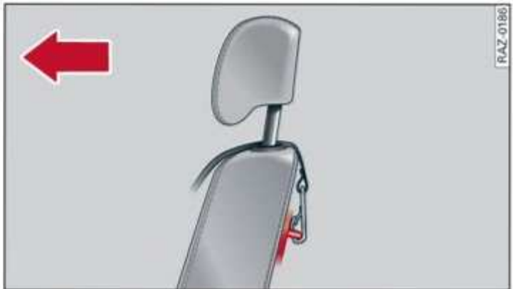
Fig. 67 Rear backrest: securing the upper belt to the top tether anchor
