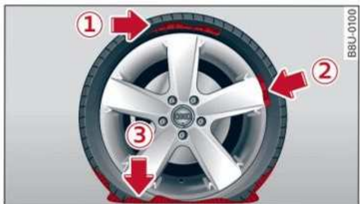
Fig. 170 Tire: tire damage that cannot be repaired
