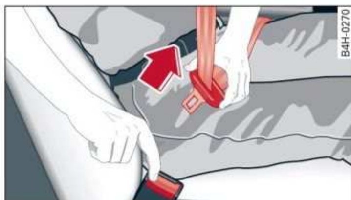
Fig. 61 Releasing the belt buckle from the belt latch
