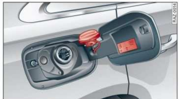
Fig. 155 Fuel filler door with attached fuel cap
