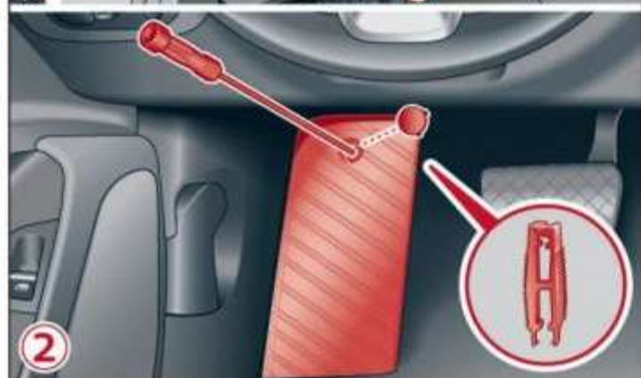
Fig. 186 Left side of the cockpit: fuse panel cover ①, driver's footwell: fuse panel cover and clip ②
