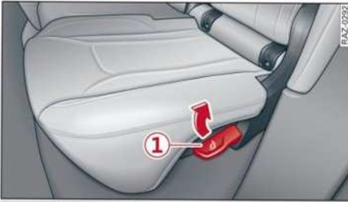
Fig. 75 Rear bench seat: release lever
