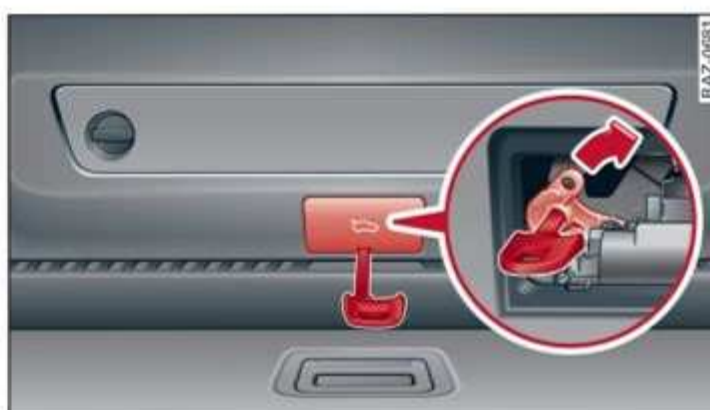
Fig. 31 Inner luggage compartment lid: access to the manual release
