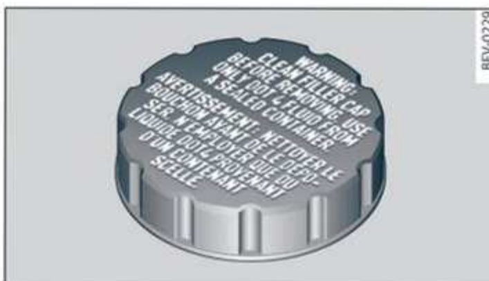
Fig. 162 Engine compartment: cap on brake fluid reservoir
