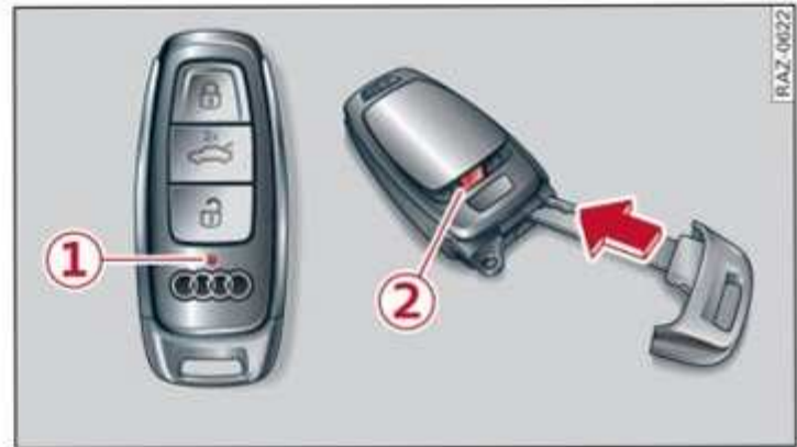
Fig. 26 Vehicle key: removing the battery holder
