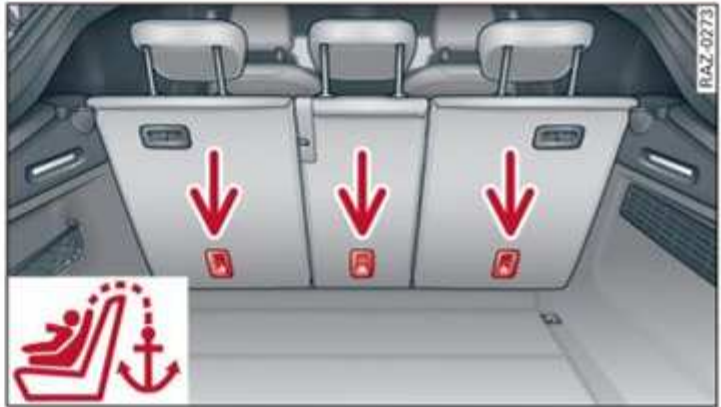
Fig. 66 Rear backrest: top tether anchors to secure a child safety seat with an upper belt
