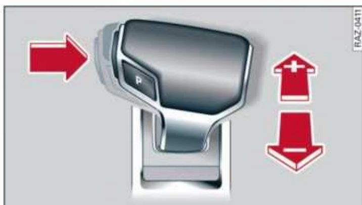
Fig. 85 Center console: shifting manually with the selector lever
