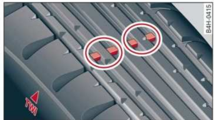
Fig. 166 Tire profile: treadwear indicator
