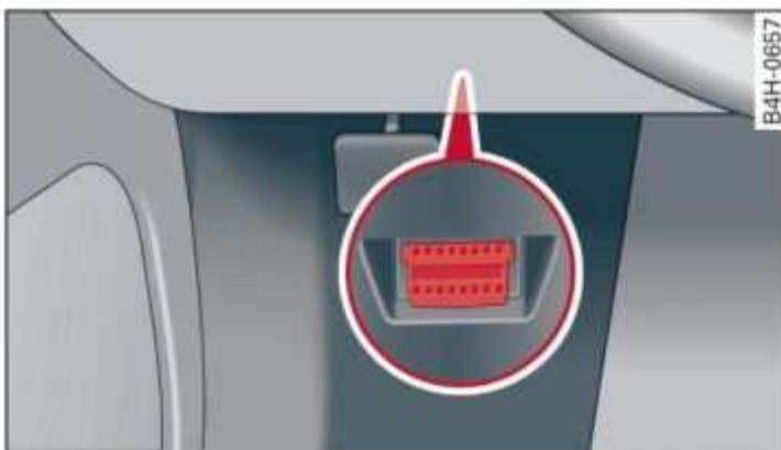
Fig. 192 Driver's side footwell: connection port for the On Board Diagnostic System (OBD)
