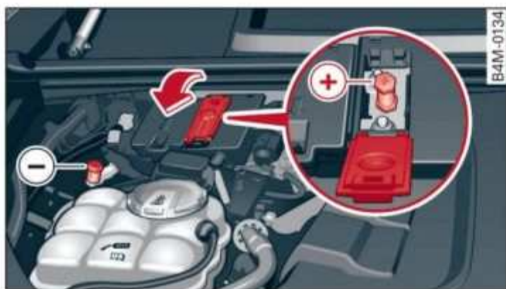
Fig. 163 Engine compartment: connectors for a charger or jump start cables
