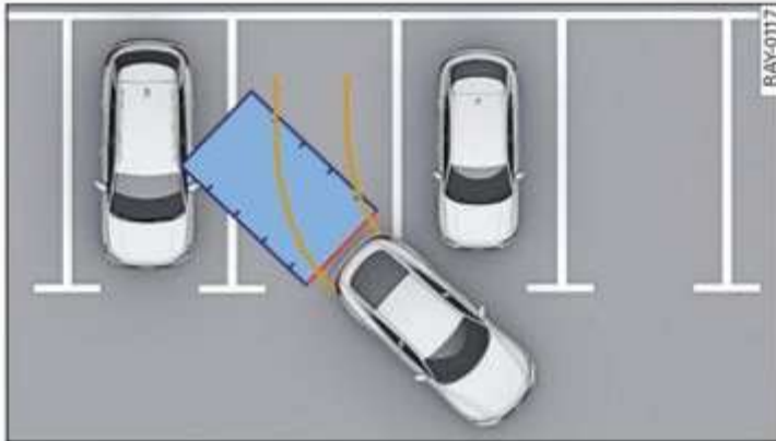
Fig. 121 Orientation line display when parking
