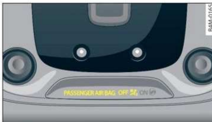
Fig. 64 Headliner: indicator light to display the status of the front passenger's airbag
