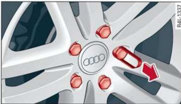
Fig. 173 Wheel: wheel bolts with caps
