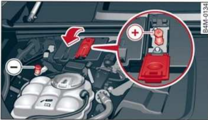
Fig. 180 Engine compartment: connectors for jump start cables or a charger
