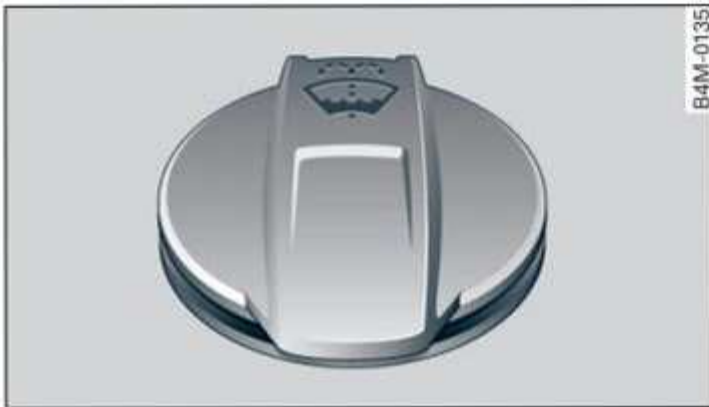
Fig. 164 Engine compartment: washer fluid reservoir cap
