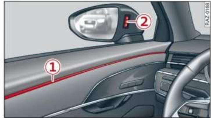
Fig. 116 Front door: warning strip
