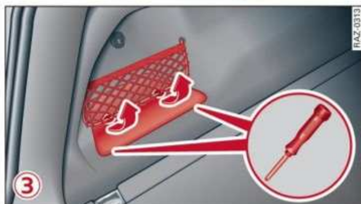
Fig. 187 Left side of the luggage compartment: fuse panel cover ③
