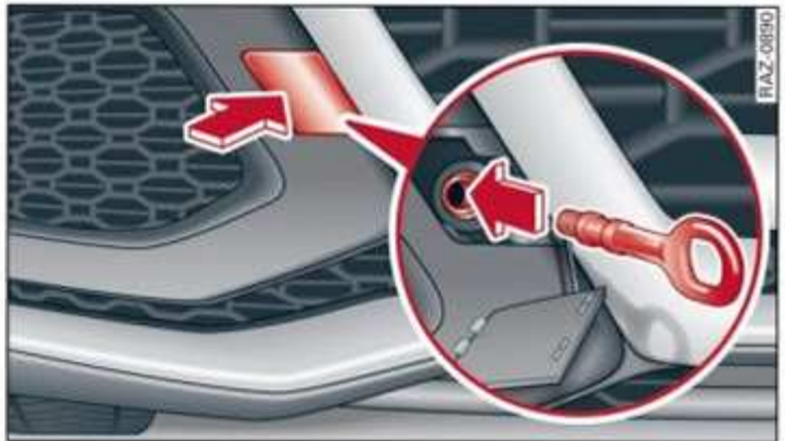
Fig. 183 Front bumper: installing the towing loop (version 2)
