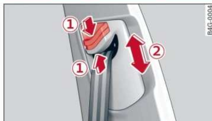
Fig. 62 Belt height adjustment for the front seats - safety belt relay
