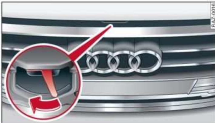
Fig. 157 Unlocked hood: lever
