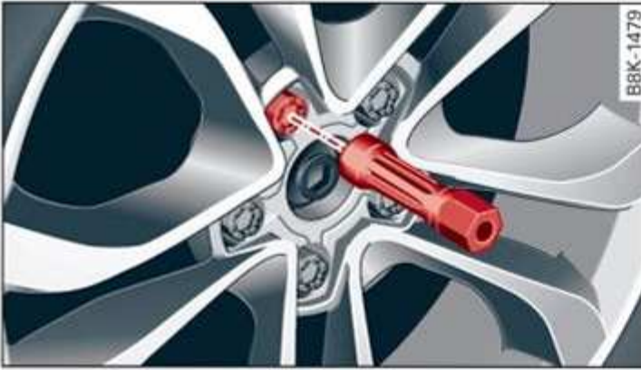
Fig. 178 Wheel: internal hex socket to turn the wheel bolts
