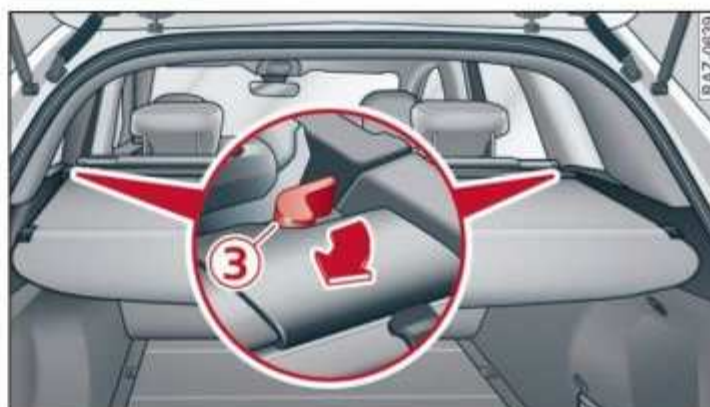
Fig. 72 Luggage compartment: removing the luggage compartment cover
