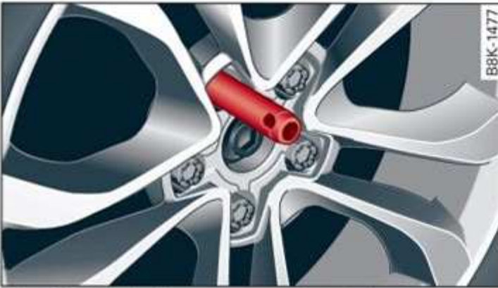
Fig. 179 Wheel: alignment pin in the top hole
