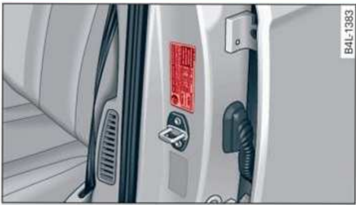
Fig. 167 Driver's side B-pillar: tire pressure label
