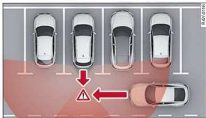
Fig. 132 Sensor detection range for rear cross-traffic assist
