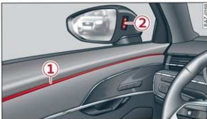
Fig. 123 Front door: warning strip
