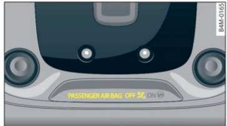
Fig. 70 Headliner: Indicator light to display the status of the front passenger's airbag
