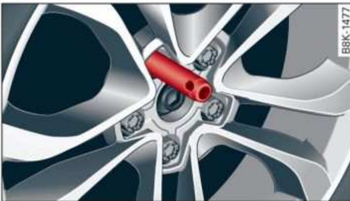
Fig. 183 Wheel: alignment pin in the top hole
