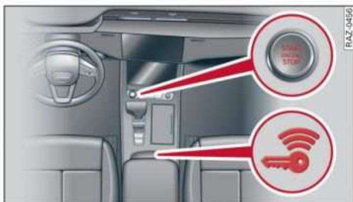
Fig. 87 Center console: starting the engine
