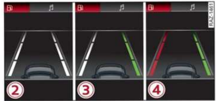
Applies to: driver assistance display without area view Fig. 119 Instrument cluster: lane departure warning
