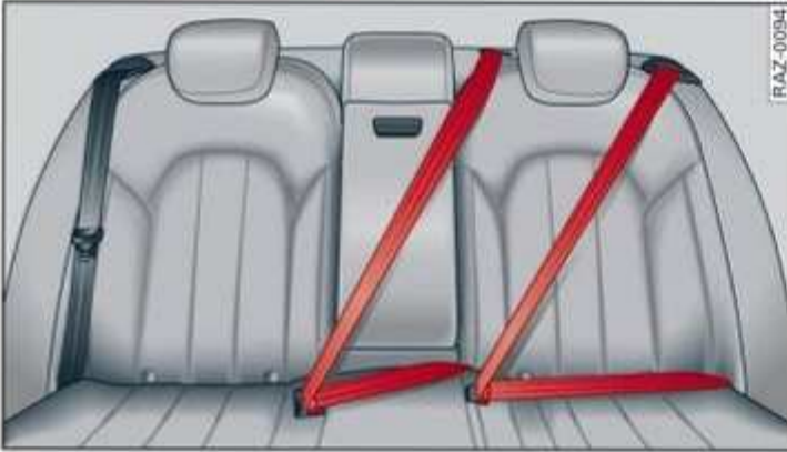
Fig. 74 Rear bench seat: securing unused safety belts
