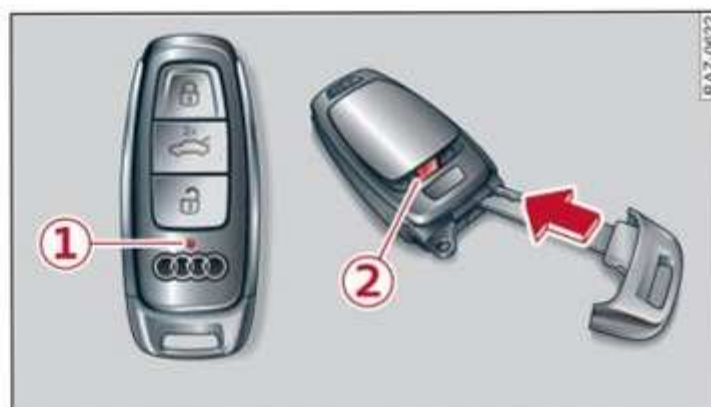
Fig. 29 Vehicle key: removing the battery holder
