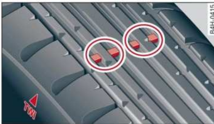
Fig. 172 Tire profile: treadwear indicator
