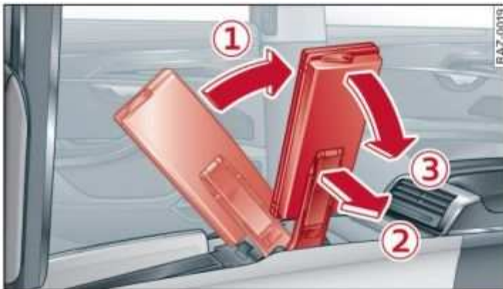
Fig. 78 Rear center console*: opening the folding tray table
