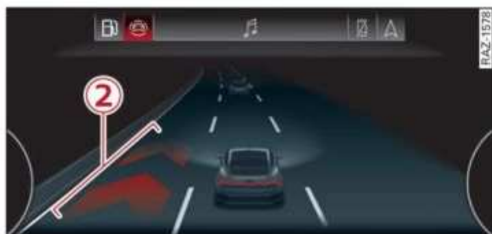
Applies to: driver assistance display with area view Fig. 121 Instrument cluster: side assist display
