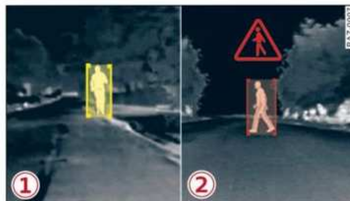
Fig. 100 Instrument cluster: pedestrian marking and warning
