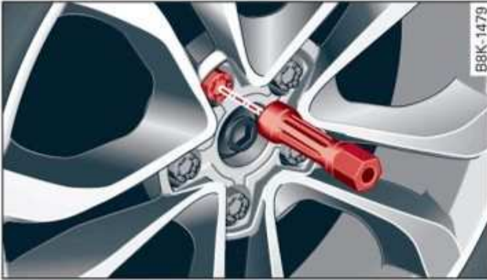
Fig. 182 Wheel: internal hex socket to turn the wheel bolts
