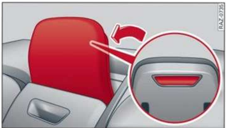
Fig. 63 Center rear seat*: folding up the head restraint
