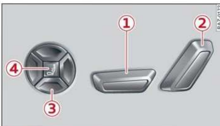
Fig. 51 Front seat: seat adjustment buttons
