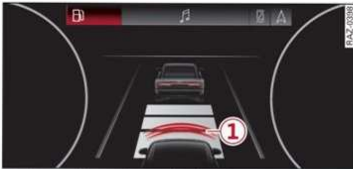
Applies to: driver assistance display without area view Fig. 113 Instrument cluster: safe start monitor
