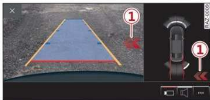
Fig. 133 Upper display: rear cross-traffic assist display
