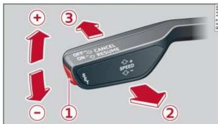
Fig. 101 Operating lever: switching the system on
