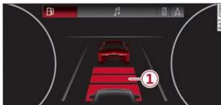
Applies to: driver assistance display without area view Fig. 108 Instrument cluster: brake intervention request
