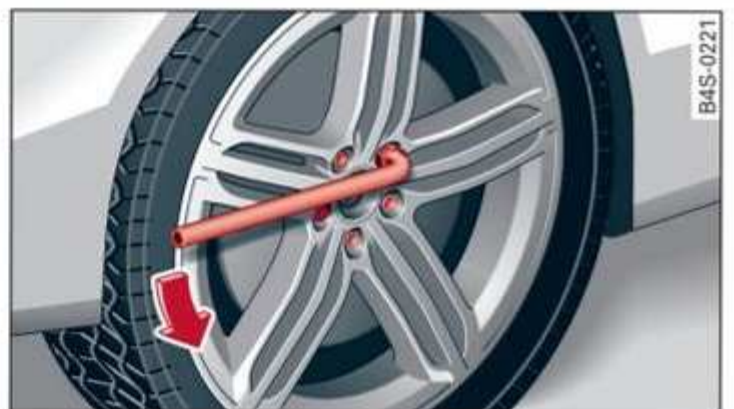
Fig. 179 Wheel: loosening the wheel bolts
