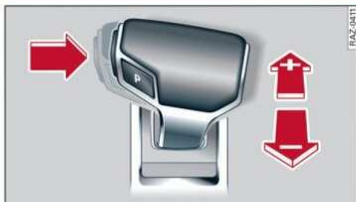
Fig. 89 Center console: shifting manually with the selector lever
