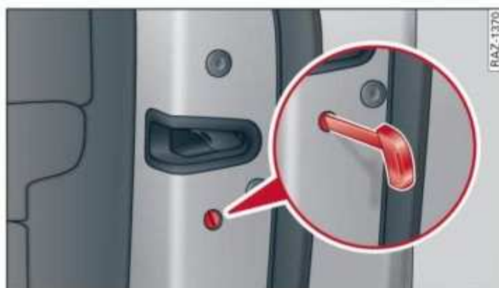
Fig. 26 Door: mechanically locking
