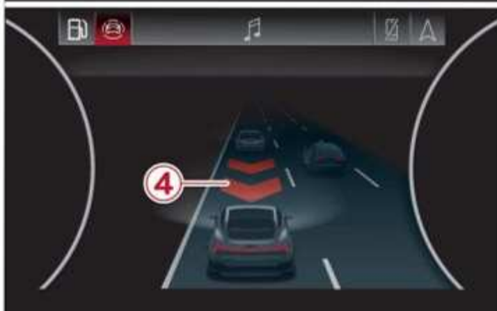
Fig. 117 Instrument cluster: distance warning with or without area view
