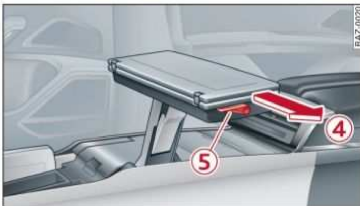
Fig. 79 Rear center console*: extending and adjusting the folding tray table
