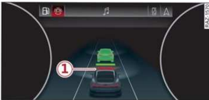
Applies to: driver assistance display with area view Fig. 114 Instrument cluster: safe start monitor
