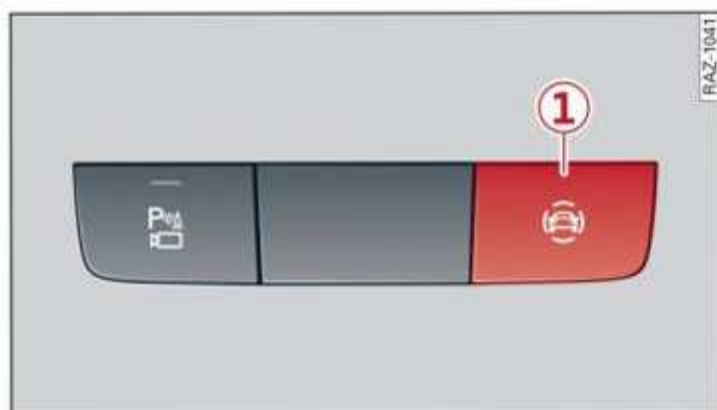
Fig. 96 Center console: driver assistance systems button
