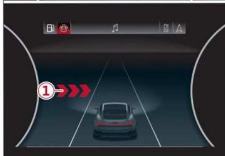
Fig. 125 Instrument cluster: intersection assistant direction display with or without area view
