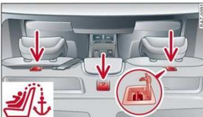
Fig. 72 Rear shelf: top tether anchors to secure a child safety seat with an upper belt
