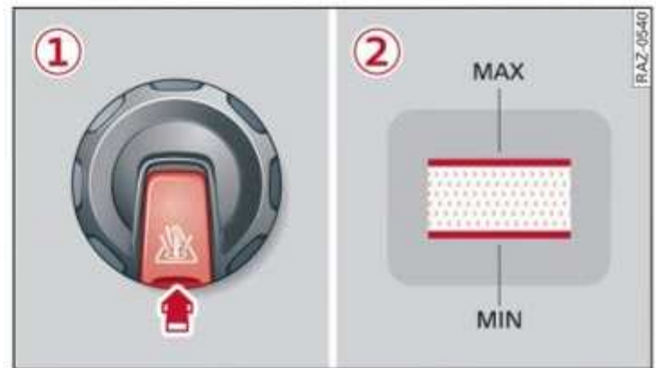
Fig. 167 Engine compartment - Coolant expansion tank (diagram): ① cover with release button; ② markings
