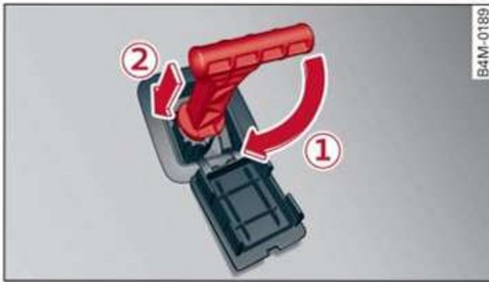
Fig. 91 Footwell: releasing the parking lock using the emergency release
