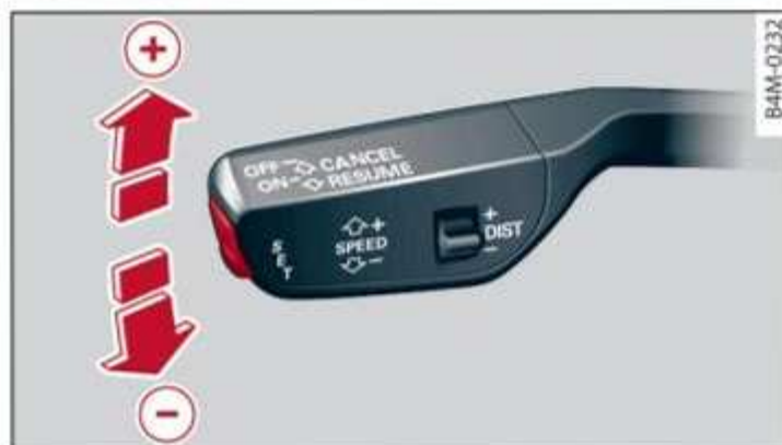
Fig. 106 Operating lever: changing the speed
