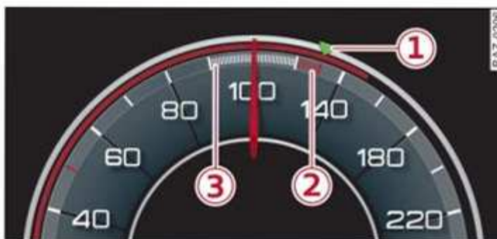
Fig. 110 Instrument cluster: speedometer: predictive control display
