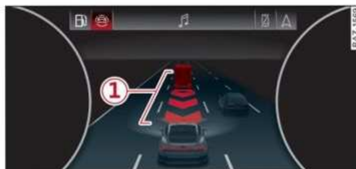
Applies to: driver assistance display with area view Fig. 109 Instrument cluster: brake intervention request
